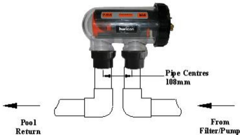
**WARNING:** It is essential that pipe work and equipment do not allow gases generated from the cell to collect and build up.
